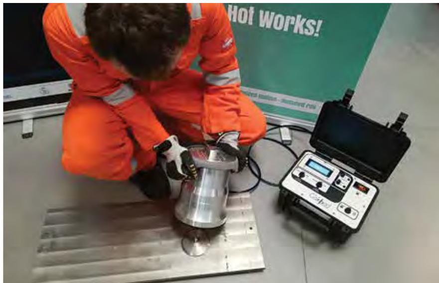
**ABOVE:** Process-controlled tooling of C-Claw. (All images courtesy Cold Pad)
